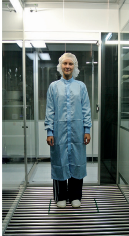
Test person in cleanroom lab coat with non-woven bouffant cap over cotton garments
