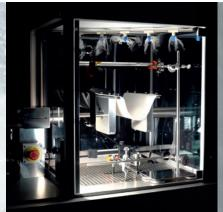
R&D: Newly developed test bench Determination of the particle emission of dry wipes with the inclusion of mechanical stress
