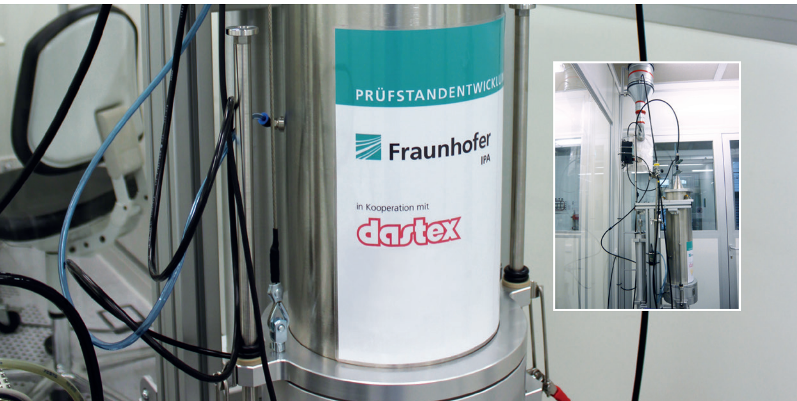
New filter test bench for cleanroom fabrics, a joint development by Dastex and Fraunhofer IPA (Stuttgart)
