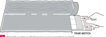
5 Open the section with the mop covers using the tear notch to pull them out. Use them within a maximum of 2 hours.
