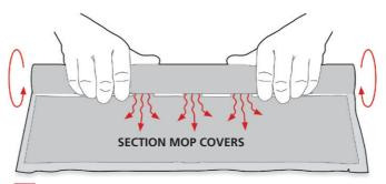
3 To ensure maximum flow of the biocide to the mop cover side, roll and compress the liquid side of the pouch to force all the liquid into the section with the mop covers.
