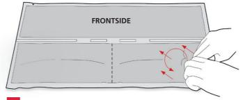
1 Place the 2-component pouch on a flat surface and roll up the right liquid section, then hold it firmly with one hand and press it with the other hand downwards, around the inner pouch section 1 to make it bursts open. Press out the content
